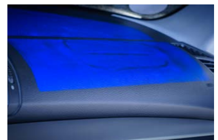
Full-surface back projection of the inspection result
